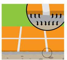
When tiling is done with a standard performance adhesive onto an impervious substrate, the adherence is much weaker resulting in tiles de-bonding from the substrate.
