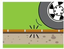
Any area of the tile that has no contact on the substrate and has voids is vulnerable when subjected to a localized load. These fragile points will let cracks and crashes of the covering.
