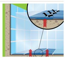
Tiling onto under floor heated systems; the tiles usually have a lower coefficient of thermal expansion. For a given temperature rise tiles will expand less than the substrate and stresses will be formed at the interface between the tile and the adhesive. At weak bonded parts, the tiles may delaminate or blow away from their base. Same rule applies for the substrates on heat transmitting systems and insulation applications.
